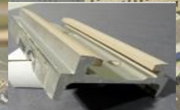
Improved coating on missile rail surfaces: 10x improved wear
