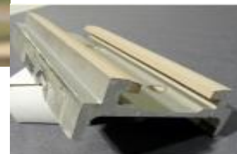
Improved coating on missile rail surfaces: 10x improved wear
