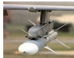
Improved coating on missile rail surfaces: 10x improved wear
